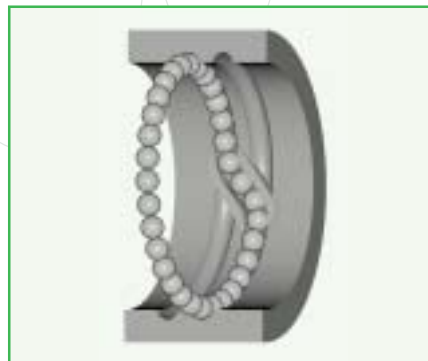
Fig 3.5 Circuit for internal return cap
